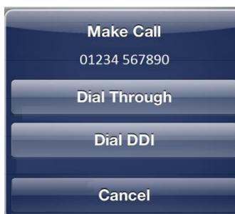
If a DDI number is associated with an extension, you can also dial the DDI number directly by pressing **Dial DDI** (instead of Dial Through). This option requires the DDI number to be preconfigured against the extension on the Xchange Server. For more information please contact your Samsung Telephone System administrator.
